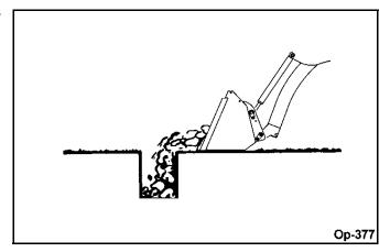
Operate tractor at right angles to ditch. Take as big a bite as tractor can handle without lugging down.
